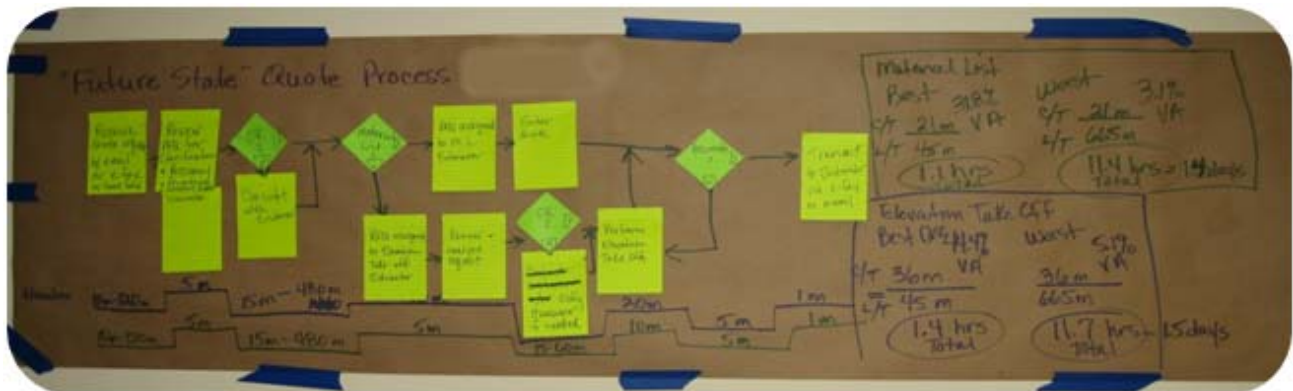
Fig 2. In the future state quote process, both value-added and non value-added times were reduced through the implementation of a new software system, leading to new baselines for value-added times of 32% (best case) and 3.1% (worst case) for material lists and 44.4% (best case) and 5.1% (worst case) for elevation take offs.
