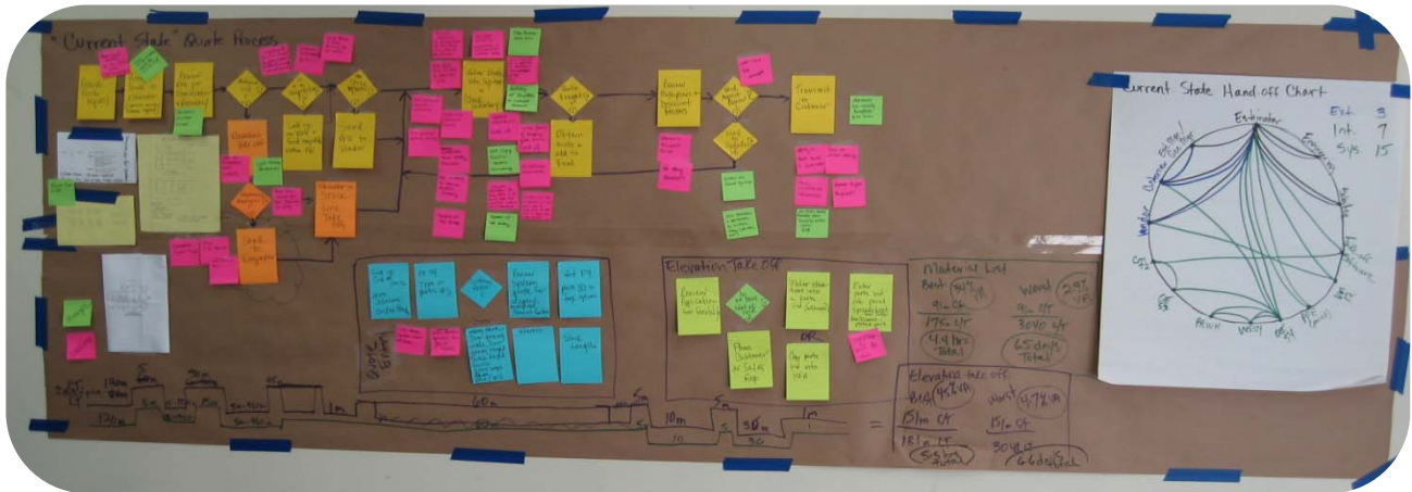
Fig 1. The current state quote process map revealed value-added times of 34% (best case) and 2.9% (worst case) for material lists and 45% (best case) and 4.7% (worst case) for elevation take offs, leaving a great deal of room for improvement.
